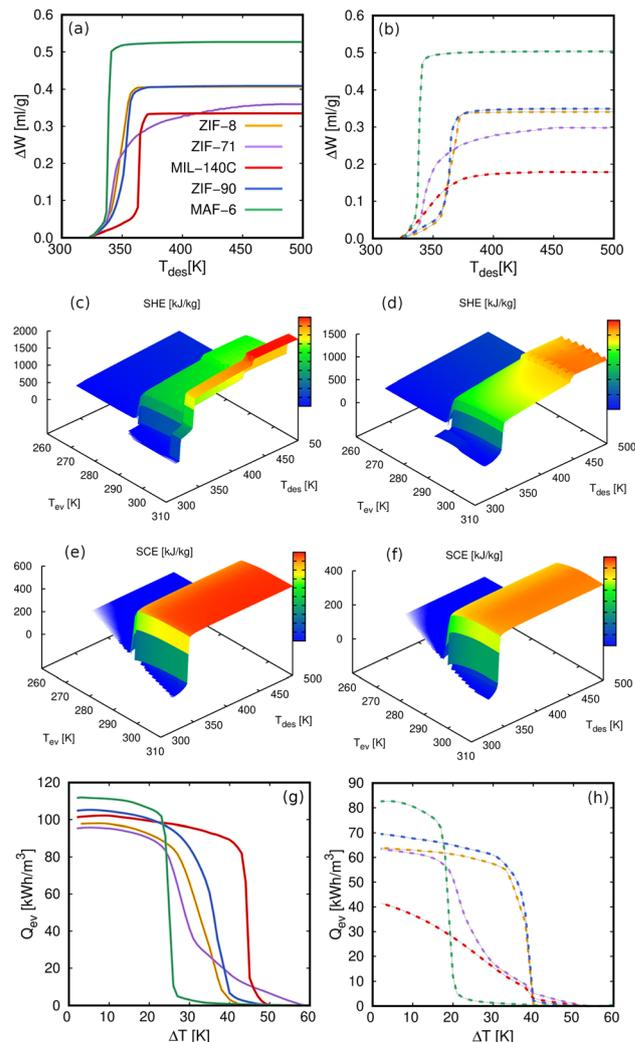
**Fig. 12** Deliverable capacity for (a) methanol and (b) ethanol as a function of the desorption temperature for  $T_{ev} = 300\text{ K}$  and  $T_{con} = 310\text{ K}$ . The SHE and SCE of (c and e) methanol and (d and f) ethanol in MAF-6 at  $T_{con} = 313\text{ K}$ .  $Q_{ev}$  as a function of temperature lift ( $T_{con} - T_{ev}$ ), for (g) methanol and (h) ethanol varying  $T_{ev}$  with  $T_{con}$  and  $T_{des}$  set to 298 K and 373 K, respectively.
