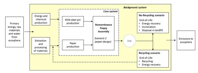
Fig. 3 Schematic of the "cradle-to-grave" system boundaries considered for scenario 2 (S2) design. \*Incineration refers to the option without energy recovery.
