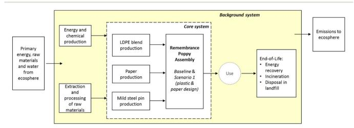
Fig. 2 Schematic of the "cradle-to-grave" system boundaries considered for baseline and scenario 1 (S1) designs. \*Incineration refers to the option without energy recovery.
