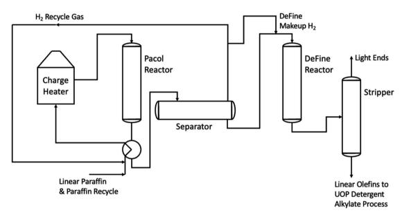
Fig. 6 UOP Pacol dehydrogenation process (adapted from Bhasin et al.).4
