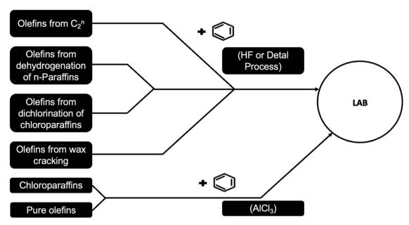
Fig. 5 The most common LAB production methods (adapted from Shokri and Karimi).<sup>3</sup>
