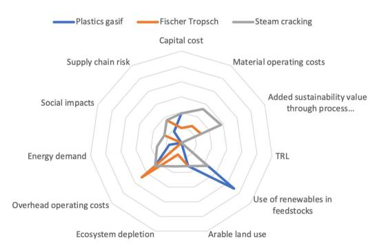
Fig. 8 Sample spider diagram showing weighted impact results for supply chain SJ, concerning the gasification and FT synthesis of plastics (axis concealed to hide discrete priority factors).
