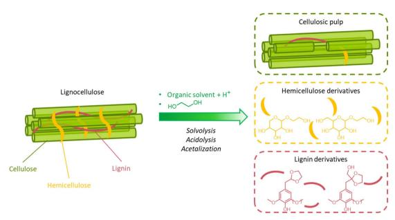
Fig. 43 Schematic outline of the DAF process for the extraction, depolymerization and stabilization of lignin (and hemicellulose) derivatives from lignocellulosic biomass *via* solvolysis/acidolysis, acidolysis, and acetalization, respectively. Note: in this example, ethylene glycol is shown as a diol, but, in general, other diols can be adopted as well. The organic solvent should be an aprotic solvent, to prevent possible condensation reactions with the diol.
