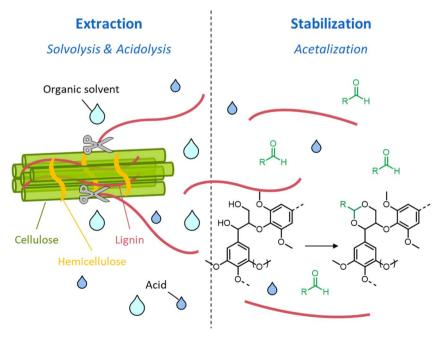
Fig. 38 Schematic representation of lignin extraction and stabilization during AAF.
