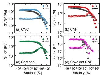
Fig. 3 Storage (closed symbols) G' and loss (open symbols) G'' moduli as a function of oscillatory strain  $\gamma$  for the four classes of gels: (a) CNC, (b) entangled CNF, (c) Carbopol, and (d) covalent CNF. Data collected with increasing and decreasing  $\gamma$  are shown in color and gray, respectively.
