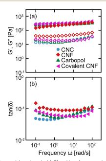
Fig. 2 (a) Storage (closed symbols) G' and loss (open symbols) G'' moduli and (b)  $tan(\delta) = G''/G'$  as a function of frequency  $\omega$  for the four classes of gels: CNC, entangled CNF, Carbopol, and covalent CNF
