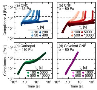
Fig. 5 Compliance  $J = \gamma/\sigma$  as a function of time at constant stress  $\sigma$  for various waiting times  $t_w$  after yielding for (a) CNC, (b) entangled CNF, (c) Carbopol, and (d) covalent CNF gels. Dashed lines indicate the creep threshold  $J^*$  used to identify the yield time  $\Delta t_{\nu}$
