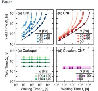
Fig. 6 Yield time  $\Delta t_v$  as a function of waiting time  $t_w$  under different applied stresses  $\sigma$  for (a) CNC, (b) entangled CNF, (c) Carbopol, and (d) covalent CNF gels. Curves are guides to the eye.
