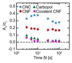
Fig. 9 Normalized hysteric area  $A_{\sigma}/\sigma_{\rm c}$  as a function of the time interval per step  $\delta t$  in flow sweeps for different gel classes.
