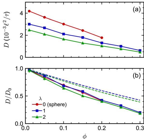
Fig. 6 (a) Long-time self-diffusion coefficient  $D$  for spherocylinders with aspect ratios  $\lambda = 1$  and 2 as a function of volume fraction  $\phi$ . The sphere data from Fig. 2 is included as a reference point with  $\lambda = 0$ . (b)  $D$  normalized by its value extrapolated to infinite dilution  $D_0$ . The dashed curves in (b) are  $D/D_0$  predicted from the fit of ref. 97.
