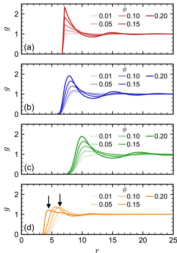
Fig. 3 Radial distribution function for (a) spheres, (b) octahedra, (c) cubes, and (d) tetrahedra at different nominal volume fractions  $\phi$ . The arrows in (d) denote signature peaks for the transition to pentagonal dipyrramids at  $0.55a_{\text{ex}}$  and  $0.75a_{\text{ex}}$ .<sup>84,85</sup>
