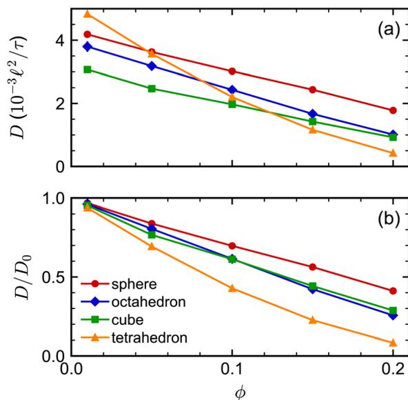
Fig. 2 (a) Long-time self-diffusion coefficient  $D$  of spheres, octahedra, cubes, and tetrahedra as a function of nominal volume fraction  $\phi$ . (b)  $D$  normalized by its value linearly extrapolated to infinite dilution  $D_0$ .
