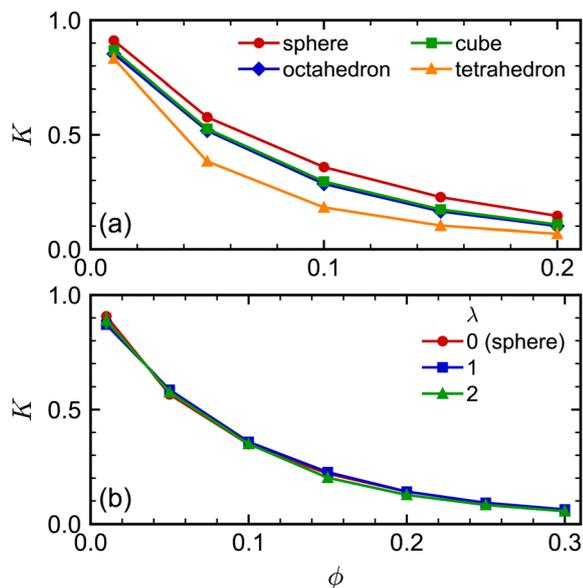
Fig. 7 Sedimentation coefficient  $K$  of (a) spheres, octahedra, cubes, and tetrahedra and (b) spherocylinders as a function of volume fraction  $\phi$ . The frame of reference used to define  $K$  is the one where the volume-averaged velocity is zero.
