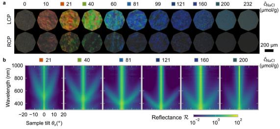
Fig. 3 (a) Polarised optical microscopy (POM) in reflection mode for photonic CNC films with increasing NaCl: CNC ratio  $\hat{c}_{NaCl}$ . Images were acquired through a left- and right-circularly polarised analyser (LCP and RCP respectively). (b) Tilt scan data for selected  $\hat{c}_{NaCl}$  values. Colour bar indicates log-scale reflectance  ${\cal R}$  normalised to a diffuse reflectance standard.
