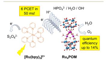
Scheme 1 Multiple and sequential proton coupled electron transfer events from a tetraruthenium polyoxometalate  $Ru_4POM$  to photogenerated  $[Ru(bpy)_3]^{3+}$  investigated in this work through laser flash photolysis, with  $HPO_4^{2-}$ ,  $H_2O$  and  $OH^-$  being responsible for proton transfer.
