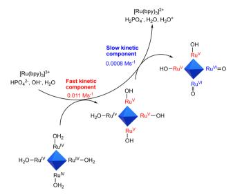
Scheme 2 Schematic representation of the accumulation of oxidation equivalents on Ru<sub>4</sub>POM through sequential PCET involving  $[Ru(bpy)_3]^{3+}$  and aqueous bases within two kinetic regimes.
