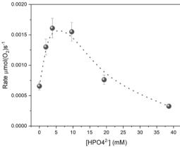
Fig. 4 (Top panel) O<sub>2</sub> evolution kinetics (see Table 2 for conditions). (Bottom panel) Plot of Rate(O<sub>2</sub>)<sub>MAX</sub> vs. the concentration of HPO<sub>4</sub><sup>2-</sup> buffer base. Error bars result from repetitive runs.
