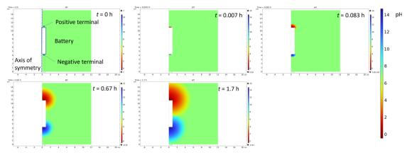
Fig. 8 Snapshots of the simulation of pH change during the chemical discharge of the Li-ion battery
