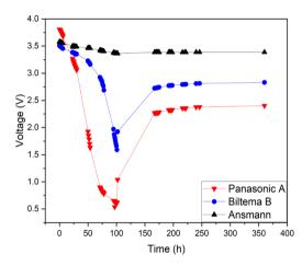
Fig. 9 Discharge behaviour of different batteries in a redox electrolyte containing a 5 wt% solution of potassium hexacyanoferrate and potassium hexacyanoferrite.
