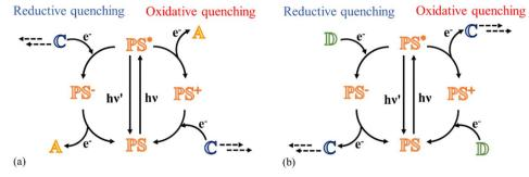
Fig. 1 Schematic of photoinduced catalysis for (a) water oxidation and (b) CO<sub>2</sub> reduction processes. Reductive and oxidative quenching mechanisms are illustrated (on the left and right side, respectively). A is the electron-acceptor species, D is the electron-donor species, PS is the photosensitizer and C represents the catalyst.
