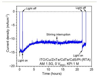
Fig. 9 Time course of the photocurrent generated by an ITO/Cu/ ZnTe/CdTe/CdS/Pt photocathode at 0 V<sub>RHE</sub> under simulated sunlight in 1 M KPi aqueous solution under 400 rpm stirring
