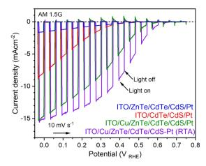
Fig. 5 Current-potential curves for ITO/CdTe/CdS/Pt, ITO/ZnTe/ CdTe/CdS/Pt, ITO/Cu/ZnTe/CdTe/CdS/Pt, and ITO/Cu/ZnTe/CdTe/ CdS/Pt (RTA) under chopped simulated sunlight. 1 M aqueous KPi solution with pH adjusted to 6.5 was used as an electrolyte. The applied potential was swept at  $+10 \text{ mV s}^{-1}$ .
