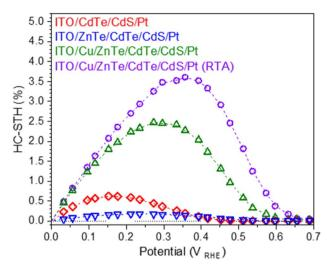
Fig. 6 HC-STH curves calculated from the current-potential curves for ITO/CdTe/CdS/Pt, ITO/ZnTe/CdTe/CdS/Pt, ITO/Cu/ZnTe/CdTe/ CdS/Pt, and ITO/Cu/ZnTe/CdTe/CdS/Pt (RTA) shown in Fig. 5.
