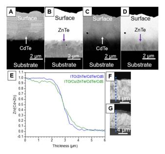
Fig. 3 Cross-sectional SEM images focused on CdTe (A and C), and those focus on ZnTe (B and D), for ITO/ZnTe/CdTe/CdS and ITO/Cu/ ZnTe/CdTe/CdS, respectively, SEM-EDS line analysis results (E), and cross-sectional SEM images with the dashed line indicating analysis performed lines for ITO/ZnTe/CdTe/CdS (F) and ITO/Cu/ZnTe/CdTe/ CdS (G).
