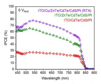
Fig. 7 IPCE spectra obtained from ITO/CdTe/CdS/Pt, ITO/ZnTe/ CdTe/CdS/Pt and ITO/Cu/ZnTe/CdTe/CdS/Pt photocathodes at 0 V<sub>RHF</sub> under monochromatic light. As an electrolyte, a 1 M aqueous KPi solution with pH adjusted to 6.5 was employed.
