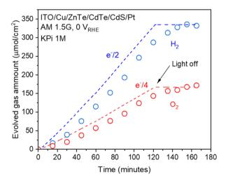
Fig. 10 Hydrogen and oxygen evolution from the ITO/Cu/ZnTe/ CdTe/CdS/Pt (RTA) photocathode under simulated sunlight in a threeelectrode configuration with an applied potential of 0 V<sub>RHF</sub>. The expected amounts of hydrogen and oxygen (denoted as e<sup>-</sup>/2 and e<sup>-</sup>/4, respectively) as calculated from the observed photocurrent are shown as dashed lines. A 1 M agueous KPi solution with pH adjusted to 6.5 with KOH was used as the electrolyte.
