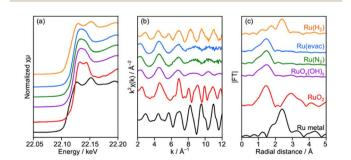
Fig. 7 (a) XANES spectra, (b) EXAFS oscillation and (c) its Fourier transforms analyzed at the Ru K-edge for Ru/CLTO prepared by the impregnation method under different heat treatment conditions.
