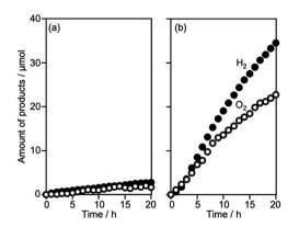
Fig. 8 Time courses of gas evolution by Z-scheme systems without the  $\text{Co(bpy)}_3^{3+/2+}$  electron shuttle; (a)  $\text{Cr}_2\text{O}_3/\text{Ru/CLTO-BiVO}_4$  and (b)  $\text{Cr}_2\text{O}_3/\text{Ru/CLTO-RGO/BiVO}_4$ . Photocatalyst: 0.05 g each; reactant solution: water, 160 mL; light source: 300 W Xe lamp ( $\lambda$  >420 nm).
