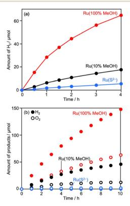
Fig. 3 Photocatalytic (a)  $H_2$  evolution and (b) Z-WS using  $Cr_2O_3$  (1.2 wt%)/Ru (0.5 wt%)/CLTO prepared under different photodeposition conditions. Photocatalyst: 0.2 g for (a) and 0.05 g each for (b); reactant solution: 10 vol% methanol for (a) and 0.1 mM Co(bpy) $_3SO_4$  for (b), 160 mL; light source: 300 W Xe lamp ( $\lambda$  >420 nm).
