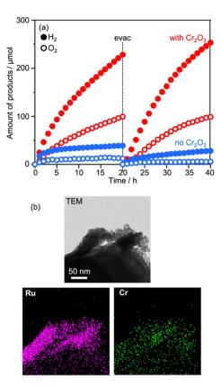
Fig. 9 (a) Influences of  $\rm Cr_2O_3$  modification on Z-WS employing Ru(100% MeOH)/CLTO. (b) TEM and element mapping images of  $\rm Cr_2O_3/Ru(100\%$  MeOH)/CLTO.
