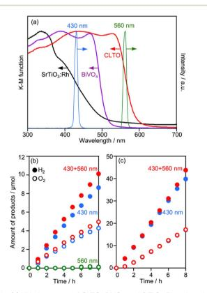
Fig. 10 (a) UV-vis spectra of CLTO, BiVO<sub>4</sub> and SrTiO<sub>3</sub>:Rh reduced by H<sub>2</sub>, and spectra of monochromatic light at 430 and 560 nm. Z-WS in  $0.1 \text{ mM } \text{Co(bpy)}_3\text{SO}_4 \text{ by (b) } \text{Cr}_2\text{O}_3/\text{Ru/CLTO-BiVO}_4 \text{ and (c) } \text{Ru/}$ SrTiO<sub>3</sub>:Rh-BiVO<sub>4</sub> systems under different irradiation conditions.
