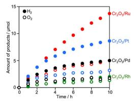
Fig. 2 Z-WS by the Cr<sub>2</sub>O<sub>3</sub>/M/CLTO-BiVO<sub>4</sub>-Co(bpy)<sub>3</sub>SO<sub>4</sub> system. Photocatalyst: 0.05 g each; reactant solution: 0.1 mM Co(bpy)<sub>3</sub>SO<sub>4</sub>, 160 mL; light source: 300 W Xe lamp ( $\lambda > 420$  nm).
