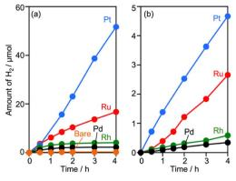
Fig. 1 Sacrificial H<sub>2</sub> evolution from a 10% methanol solution over (a) M (0.05 wt%)/CLTO and (b)  $\text{Cr}_2\text{O}_3(1.2 \text{ wt\%})/\text{M}(0.05 \text{ wt\%})/\text{CLTO}$ . Photocatalyst: 0.3 g for (a) and 0.2 g for (b); reactant solution: 10% methanol solution, 160 mL; light source: 300 W Xe lamp ( $\lambda$  >420 nm).
