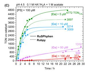
Fig. 2 Photocatalytic hydrogen production as a function of time in TON<sub>Cat</sub> under visible light irradiation (400–700 nm) from deaerated aqueous solutions (5 mL) of (A and B) NaHA (0.55 M) and  $H_2A$  (0.55 M) at pH 4.0 and (C) of NaHA (0.0714 M), H<sub>2</sub>A (0.0286 M) and 1 M acetate buffer at pH 4.5, in the presence of a PS, RuSPhphen or Rubpy and the Co catalyst at various concentrations.
