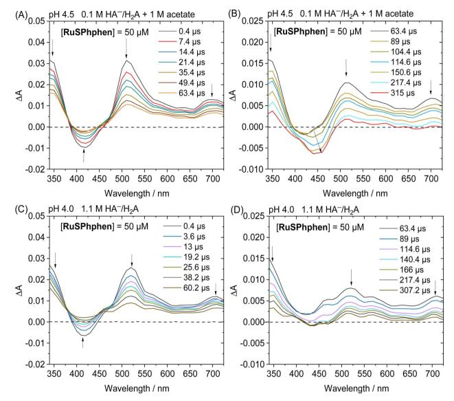
Fig. 6 Transient absorption spectra after laser excitation ( $\lambda = 462$  nm) of (A and B) a deaerated aqueous solution of 1 M acetate buffer and NaHA/  $H_2A$  (0.1 M) at pH 4.5 containing RuSPhphen (50  $\mu$ M) within the time ranges 0.4–63.4  $\mu$ s (A) and 63.4–315  $\mu$ s (B), and (C and D) a deaerated aqueous solution at pH 4.0 containing NaHA/H<sub>2</sub>A (1.1 M) and RuSPhphen (50 μM) within the time ranges 0.4–60.2 μs (C) and 63.4–307.2 μs (D); optical pathlength = 1 cm.
