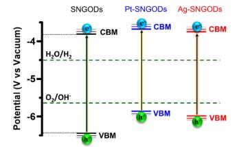
Fig. 2 Electronic-energy level diagrams of the SNGODs, Pt-SNGODs, and Ag-SNGODs in relation to the levels for H2 and O2 evolution reactions (HER and OER) in an aqueous solution of pH = 9
