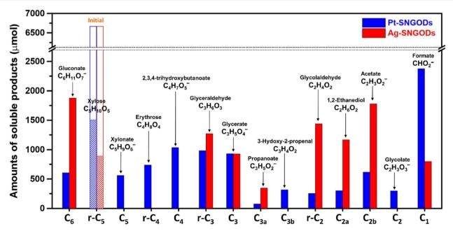
Product compositions in the liquid phase after the photocatalytic reforming of xylose for 72 h.
