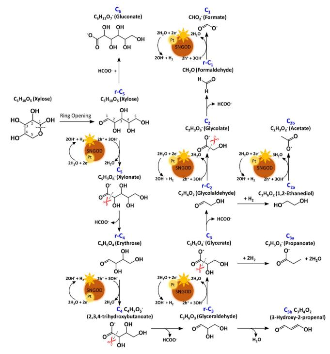
Proposed mechanism of photocatalytic reforming of xylose over Pt-SNGODs.
