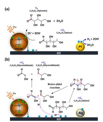
Fig. 8 The charge distributions of the SNGODs when associated with different co-catalysts. (a) Pt co-catalyst for oxidative xylose reforming (Pt-SNGODs were active in consuming photogenerated electrons for H<sub>2</sub> evolution). (b) Ag co-catalyst for retro-aldol reaction (Ag-SNGODs were less effective in HER)
