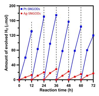
Fig. 3 Evolution of H<sub>2</sub> from the xylose solutions containing Pt-SNGODs and Ag-SNGODs under simulated solar irradiation (AM 1.5, 100 mW cm<sup>-2</sup>).
