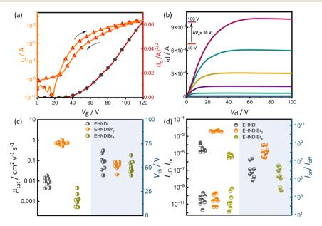
Fig. 3 OFET (a) transfer curve and (b) output curves for the EHNDIBr<sub>2</sub> thin film. (c)  $\mu_{sat}$  (left) and  $V_{th}$  (right) variations of EHNDI, EHNDIBr<sub>2</sub>, and EHNDIBr<sub>4</sub> devices. (d) Ion (top left),  $I_{off}$  (bottom left), and  $I_{on}/I_{off}$  (right) variations of EHNDI, EHNDIBr<sub>2</sub>, and EHNDIBr<sub>4</sub> devices.
