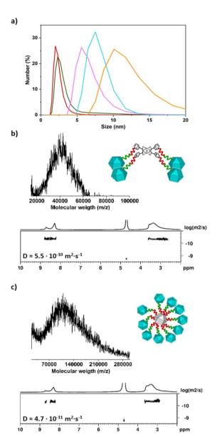
Fig. 3 (a) DLS spectra illustrating the differences in particle size (hydrodynamic-diameter) among the deprotected (N<sub>3</sub>)<sub>1</sub>-RhMOP (green), the deprotected (alkyne)<sub>1</sub>-RhMOP (red), the MOP-dimer (violet), the MOP-tetramer (cyan) and the MOP-satellite (orange). (b and c) MALDI-TOF spectra (top) and DOSY-NMR spectra (bottom) of MOP-tetramer (b) and MOP-satellite (c).
