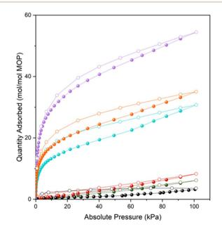
Fig. 4 Isotherms of CO<sub>2</sub>-adsorption at 195 K for the deprotected  $(N_3)_1$ -RhMOP (green), the deprotected (alkyne)<sub>1</sub>-RhMOP (red), the (alkyne)<sub>24</sub>-RhMOP (black), the MOP-dimer (purple), the MOP-tetramer (blue), and the MOP-satellite (orange).
