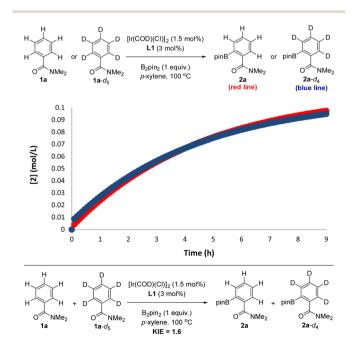
Fig. 5 Kinetic isotope effect (KIE) experiments relevant for mechanistic considerations: from two parallel reactions (top) and from an intermolecular competition (bottom).
