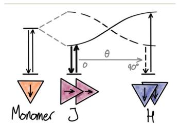
Fig. 1 Kasha's exciton model for dimers. Relative orientation as a function of the angle  $(\theta)$  between the transition dipole moments of dyes generating J- and H-aggregates with new electronic transitions.
