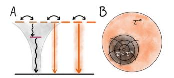
Fig. 2 Quenching by trap states. (A) Schematic state diagram with indication of energy migration between multiple similar dyes in the NPs. Presence of a dark trap state leads to full or partial quenching of many nearby dyes. (B) Illustration of the impact of a trap state able to quench a large volume of the NPs and result in shortened multi-exponential lifetimes.
