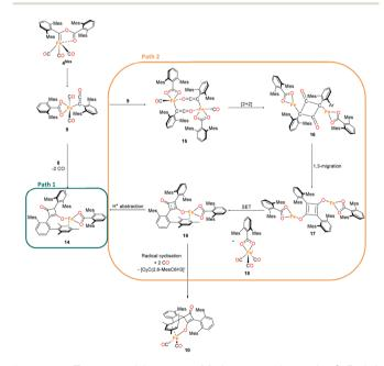
Scheme 4 Two potential routes to 14 via proposed complex 9. Path 1 forms 14 via a [2 + 2] cycloaddition of 8 and 9. Path 2 forms 14 through dimerization of 9 then a [2 + 2] cyclisation, followed by 1,3 migration and a single electron transfer, giving 18 and 19. Path 2 also has the potential to form decomposition complex 10 via radical cyclisation of 19
