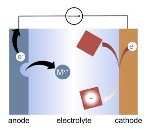
Fig. 1 Sacrificial metal anodes enable reductive electrosynthesis by charge-balancing the target reductive reactions at the cathode. During a reductive reaction, the metal sacrificial anode is oxidized, releasing metal cations into solution
