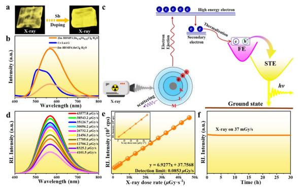
Fig. 5 X-ray scintillation performance of (Im-BDMPA)In<sub>1-x</sub>Sb<sub>x</sub>Cl<sub>6</sub>·H<sub>2</sub>O: (a) photo images of bulk crystals under X-ray irradiation; (b) RL spectra under 30 kV X-ray excitation; (c) proposed radioluminescence mechanism; (d) X-ray dose rate dependent RL emission spectra; (e) linear dependence of RL emission intensity vs. X-ray dose rate; (f) monitored RL emission intensity under continuous X-ray irradiation.
