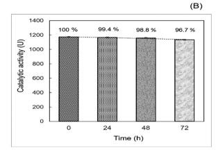
Fig. 3 (A) Catalytic activity (U) of LAR determined in the acylation of n-propanol with LA in the solvent free system at 55 °C, and in ChCl: Glc: H2O (1:1:1) and (2:1:1) R-NADESs, at 70 °C; (B) thermal stability of LAR in the ChCl:Glc:H2O (2:1:1) R-NADES, at 70 °C, assayed for the esterification of n-propanol with LA at 1:1 molar ratio.
