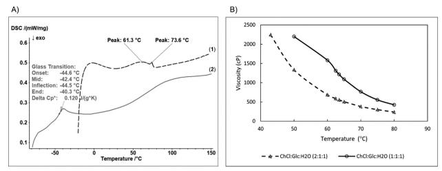
Fig. 1 (A) DSC thermograms and (B) viscosity of ChCl: Glc: H<sub>2</sub>O (1:1:1) and (2:1:1) eutectic mixtures.
