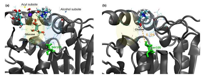
Fig. 5 Graphical representation of (a) the entrance event of glucose and (b) the particle entrance of choline in the catalytic pocket obtained from the MD trajectories of CalB in the R-NADES ChCl: Glc: H2O (2:1:1).
