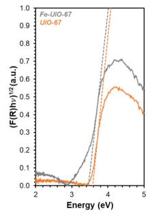
Fig. 7 DR-UV-vis data for Fe-UiO-67 (gray) and UiO-67 (orange) with K-M transformation applied. Dashed lines represent tangent lines to the rise in absorption peak for BGE calculation.
