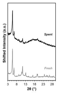
Fig. 10 XRD patterns for fresh Fe-UiO-67 (gray) and Fe-UiO-67 recovered from reaction with oxidant and UV light and solvent exchanged with acetone prior to 343 K heating (black, scaled up 1.6×).
