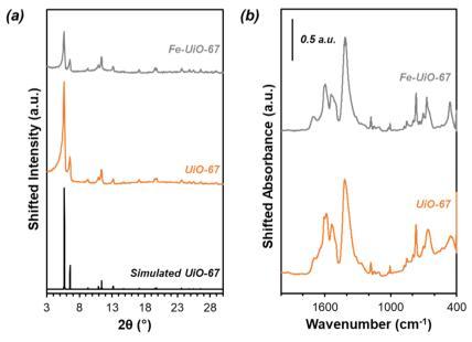
Fig. 2 (a) UiO-67 and Fe-UiO-67 experimental (orange and gray, respectively) and simulated (black) XRD patterns. Fe-UiO-67 intensity scaled up 2.5×. (b) Ex situ FT-IR absorbance spectra for synthesized UiO-67 and Fe-UiO-67. Fe-UiO-67 absorbance scaled down 0.35×.
