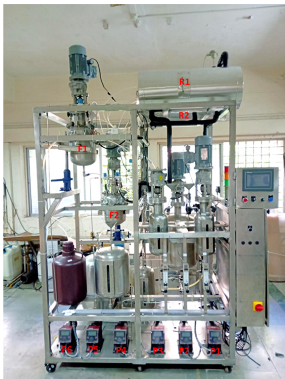
Fig. 1 Photograph of the mesoporous silica pilot plant for continuous production at a capacity of 1 kg per day. (P1 to P6) pumps, (R1, R2) helical coiled tubular reactor, and (F1, F2) two stage continuous filtration unit.
