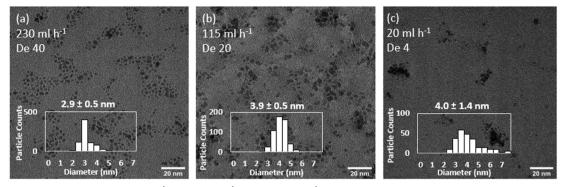
Fig. 4 Effect of total flowrate of (a) 230 ml h<sup>-1</sup>, (b) 115 ml h<sup>-1</sup> and (c) 20 ml h<sup>-1</sup> on the size and distribution of continuously synthesised Ru NPs. Representative TEM images. Experiments 1-3, Table 3.
