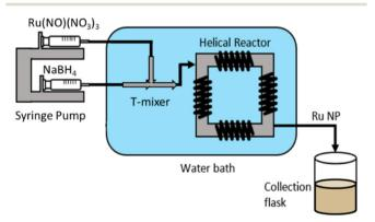
Fig. 1 Ru NP continuous reactor set up: two syringe pumps control flowrates of Ru(NO)(NO<sub>3</sub>)<sub>3</sub> and NaBH<sub>4</sub> solutions. Reactants were mixed with a T-mixer in crossflow configuration and the resulting solution passes through the coiled flow inverter reactor (CFIR).
