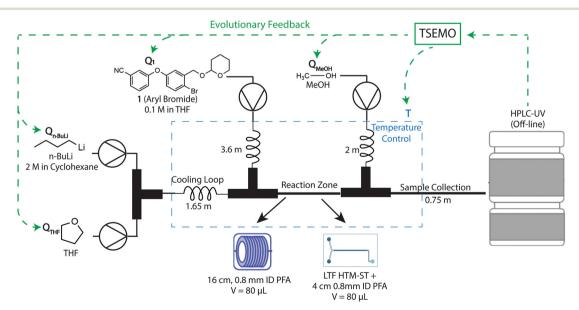
Fig. 1 A schematic representation of rector setup to perform machine learning-driven optimization of the lithium-halogen exchange of reaction given in Scheme 1b
