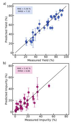
Fig. 6 Yield (a) and impurity (b) predictions of 30 experimental conditions unseen by the Gaussian process (GP) surrogate model of the first optimization campaign (Fig. 2). The mean (data points) and the standard deviation (error bars) of the predictions were calculated from the average of 1000 samples drawn from the GPs. Black solid line represents the parity line.
