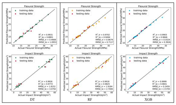
Fig. 2 Parity plots of DT, RF, and XGB models using structural characteristics to predict mechanical properties; the reference line (v = x)represents perfect prediction alignment between actual and predicted values.
