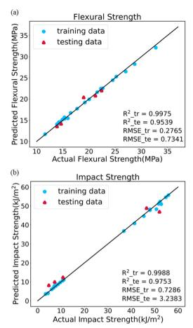
Fig. 9 Parity plots of XGB using process conditions to predict two mechanical properties: (a) FS and (b) IS.
