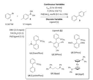
Scheme 2 Optimisation parameters for the exemplar Suzuki-Miyaura reaction between bromobenzene 4-methylphenylboronic acid 2.
