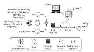
Scheme 3 Schematic of the self-optimising continuous flow reactor.
