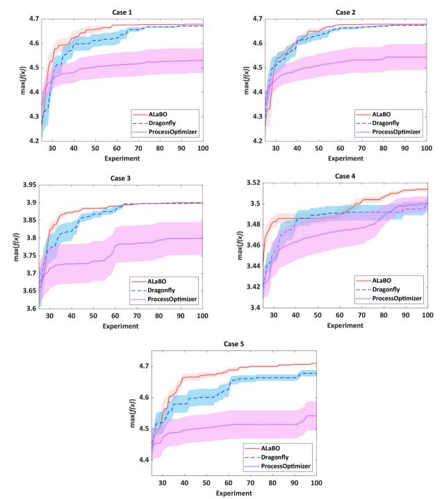
Fig. 1 Optimisation progress plots comparing algorithm performance for each of the catalytic case study simulations. Plots show the average running maxima and 95% confidence intervals across 10 separate runs with different LHC initialisation conditions.
