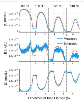
Fig. 5 Results for Pd/Al<sub>2</sub>O<sub>3</sub> at 80-140 °C. Simulated (orange) values compared with the measured (blue) values.
