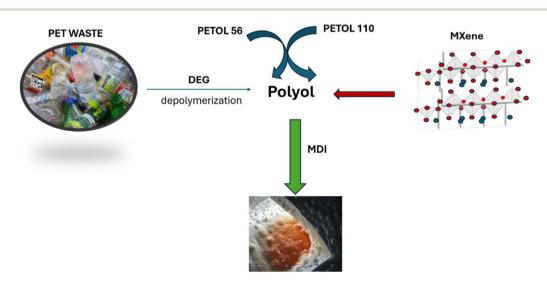
Scheme 1 The synthesis of the PUR foam filled with MXenes.
