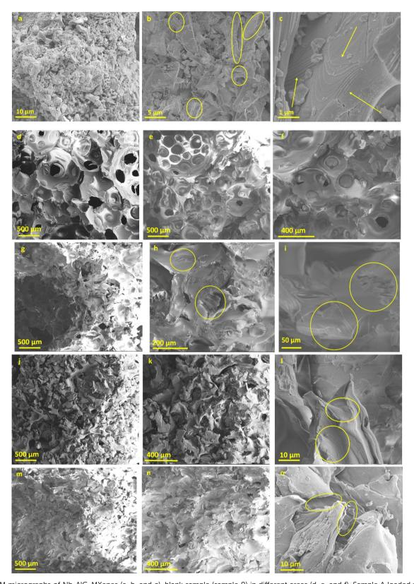
Fig. 2 SEM micrographs of  $Nb_2AlC$ -MXenes (a, b, and c), blank sample (sample 0) in different areas (d, e, and f), Sample A loaded with 0.3 g MXenes (g, h, and i), Sample B loaded with 0.5 g MXenes (j, k, and l), respectively Sample C loaded with 0.7 g MXenes (m, n, and o); the yellow arrows indicate detailed micrographs of the folded MXenes (image c), while the yellow circles evidenced the presence of exfoliated MXenes embedded in the walls of the PUR foams (detail images i, l, and o).
