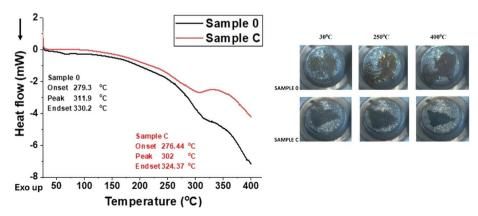
Fig. 9 DSC and optical microscopy for the samples at different temperatures.
