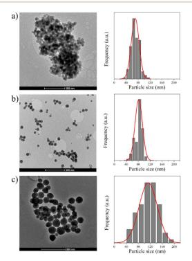
Fig. 3 TEM images of (a) MCM-41, (b) MCM-41@Ch and (c) MCM-41@Ch@DnsGly and their particle size distribution histograms.
