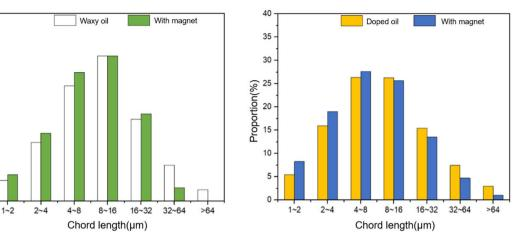
(a) Size distribution of wax crystals in the undoped waxy oil before and after magnetic treatment
