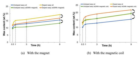
Fig. 7 Wax content in the deposition layer with the magnet or magnetic coil.
