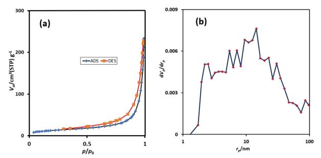
Fig. 4 The N<sub>2</sub> adsorption-desorption isotherms of urea-rich POP (a) and pore size distribution curves of urea-rich POP (b).
