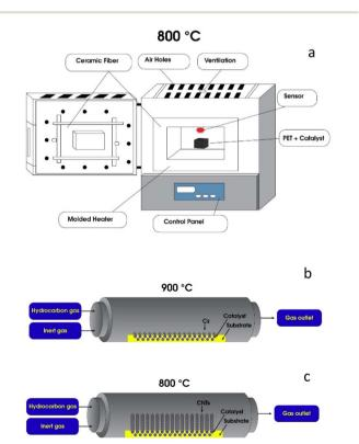
Fig. 1 Schematic illustration of catalytic fabrication of graphene (a), synthesis of carbon spheres (b), and fabrication carbon nanotubes (c).
