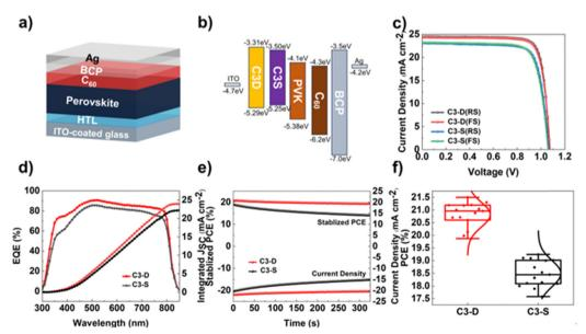
Fig. 5 (a) Device structure diagram; (b) diagram of the energy levels; (c) J-V curves measured by forward and reverse scans of the champion devices; (d) EQE spectrum and integrated short-circuit current density; (e) stability output curves at the maximum power point of the devices; and (f) the PCE statistics of devices.
