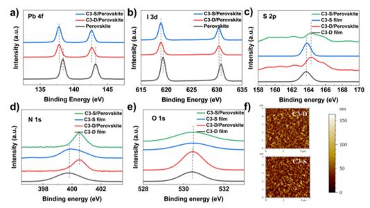
Fig. 3 XPS spectra of (a) Pb 3d, (b) I 3d, (c) S 2p, (d) N 1s and (e) O 1s for C3-D and C3-S deposited on ITO with different thickness; and (f) AFM images of C3-D and C3-S films.
