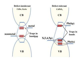
Fig. 2 Schematic representation of the electronic band structure of typical defect-intolerant semiconductors (CdSe, GaAs) and in lead halide perovskite (CsPbX<sub>3</sub>).
