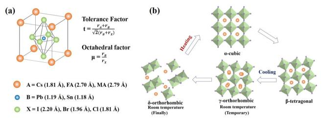
Fig. 1 (a) A cubic perovskite crystal structure (α-phase) showing flexibility in the choice of cation (A), metal (B), and anion (X), whose ionic radii are shown. (b) Schematic presentation of the structural phase transition of various polymorphs of CsPbI<sub>3</sub> as a function of temperature.
