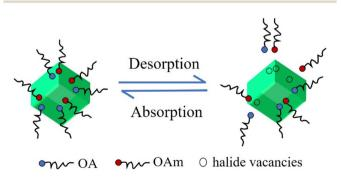
Fig. 5 Schematic representation of the dynamic surface stabilization in CsPbX<sub>3</sub> QDs.
