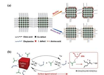
Fig. 14 (a) Schematic illustration of the changes on the PQD surface with conventional MeOAc rinsing and dual-passivation ligands before and after ligand exchange. Reproduced with permission from ref. 141. Copyright 2020, Wiley-VCH. (b) Schematic representation of the PQD dynamic surface stabilization and the ligand removal process assisted by DPA. Reproduced with permission from ref. 142. Copyright 2020, Wiley-VCH.
