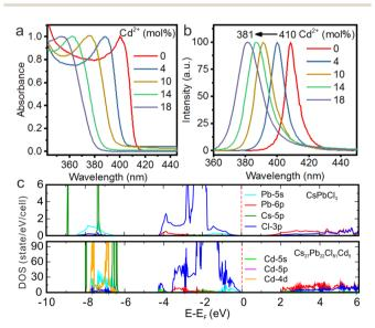
Fig. 9 (a) Absorption and (b) PL spectra for the pure CsPbCl<sub>3</sub> and CsPbCl<sub>3</sub>:Cd<sup>2+</sup> NCs. (c) Calculated density of states for pure CsPbCl<sub>3</sub> and CsPbCl<sub>3</sub>:Cd<sup>2+</sup>. Reproduced with permission from ref. 89. Copyright 2021, Wiley-VCH Verlag GmbH l Co. KGaA, Weinheim
