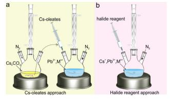
Fig. 2 (a) Schematic illustration for the synthesis of transition metal iondoped cesium lead halide perovskite NCs via hot injection method based on (a) Cs-oleates approach and (b) halide reagent approach.
