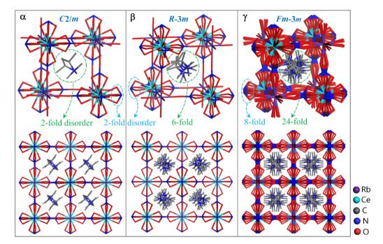
Fig. 2 Cage units and packing diagrams of 2 at 173 K ( $\alpha$  phase), 273 K ( $\beta$  phase), and 293 K ( $\gamma$  phase), respectively. The (i-PrNHMe<sub>2</sub>)<sup>+</sup> and NO<sub>3</sub><sup>-</sup> ions exhibit varying degrees of disorder in all phases. H atoms are omitted for clarity.
