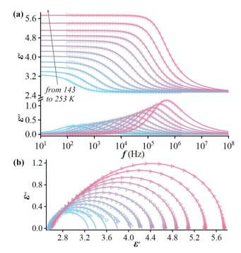
Fig. 4 Frequency-dependent  $\varepsilon'$  and  $\varepsilon''$  for 2 at selected temperatures from 143 to 253 K in an increasing step of 10 K (a), and the Cole-Cole diagrams are plotted as a series of arcs to show the relationship between  $\varepsilon'$  and  $\varepsilon''$  (b). Solid curves represent the fit of the experimental data to the Havriliak-Negami equation.
