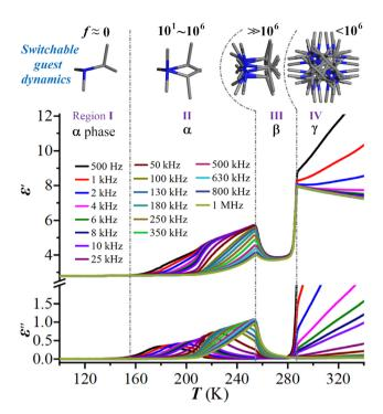
Fig. 3 Temperature-dependent  $\varepsilon'$  and  $\varepsilon''$  of 2 at various AC frequencies and the related switchable quest dynamics.
