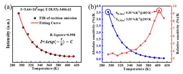
Fig. 5 (a) Plot of intensity at different temperatures with nonlinear fitting curves; (b)  $S_A$  curve and  $S_R$  curve as a function of temperature.
