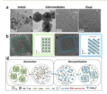
Fig. 4 Transient phases in the conversion of CsPbBr $_3$  to Cs $_4$ PbBr $_6$ : (a) TEM images of the initial Br perovskite NCs and of intermediates upon conversion to the final Cs $_4$ PbBr $_6$  product. TEM images and atomic model (b) of cubic CsPbBr $_3$  (c) and of rhombohedral Cs $_4$ PbBr $_6$ NCs. (d) Schematic of the proposed dissolution–recrystallization transformation mechanism.
