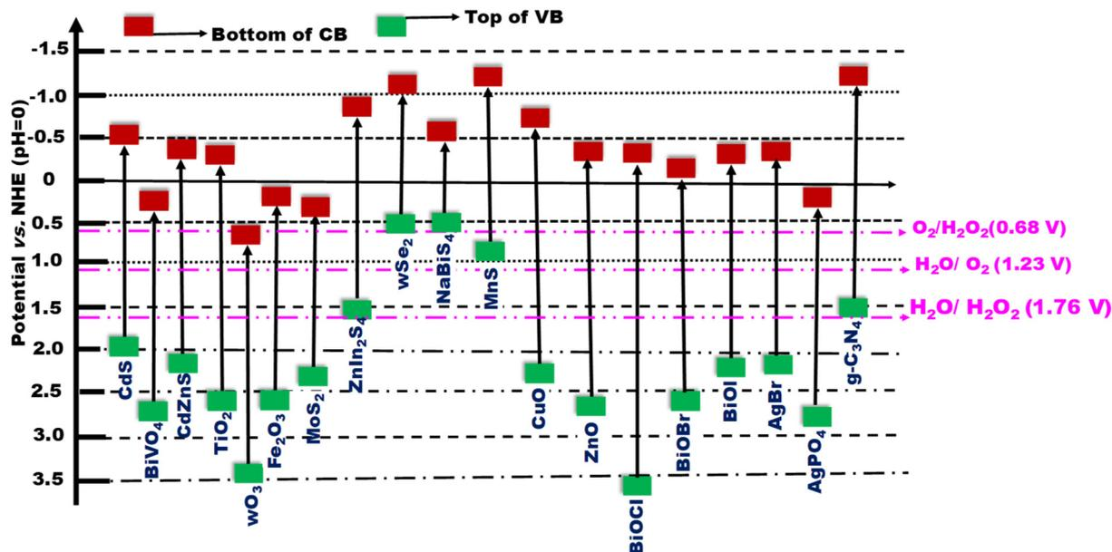
Fig. 10 Band structures of various semiconductors frequently utilized to create Z- or S-scheme heterojunctions with g-C<sub>3</sub>N<sub>4</sub>.
