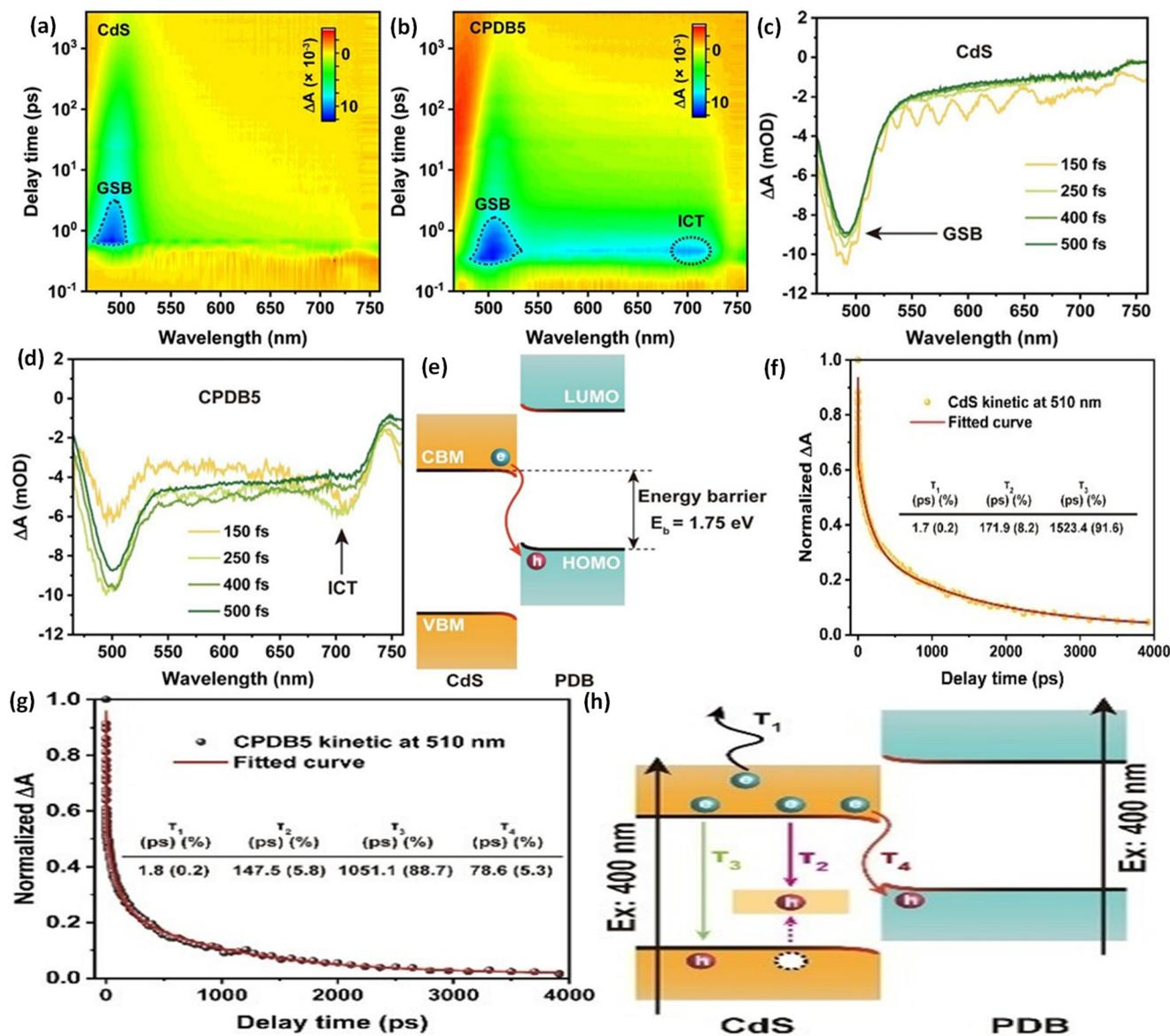
**Fig. 16** 2D mapping of TA spectra for (a) pristine CdS and (b) CPDB5 photocatalyst. TAS signals of (c) CdS and (d) CPDB photocatalyst over fs–ns timescales. (e) Depiction of the energy gap between the CBM of CdS and the HOMO level of PDB. Normalized decay kinetics of (f) CdS and (g) CPDB5 measured at a wavelength of 510 nm. (h) Decay routes for photoinduced electrons within CdS and CPDB photocatalysts. The figures are adapted with permission from ref. 169. Copyright 2023, Wiley-VCH.
