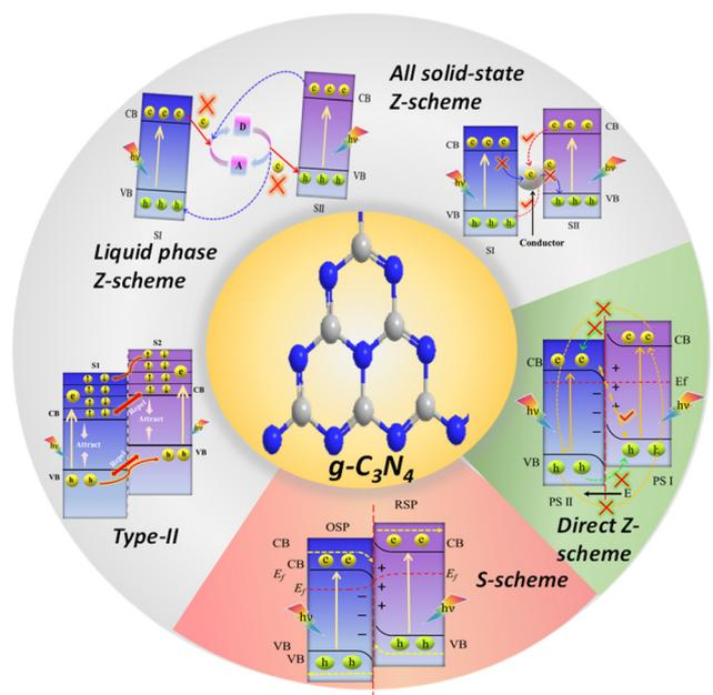
Fig. 3 Illustration of charge transfer mechanisms in different  $g\text{-C}_3\text{N}_4$ -based heterojunctions.
