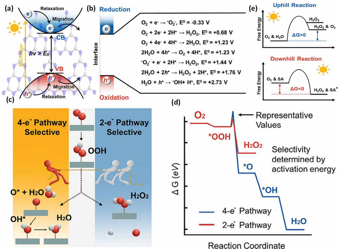
**Fig. 22** Illustrations of various stages of (a) photoexcitation and transfer of charge carriers. (b) Surface redox reaction processes relevant to solar H<sub>2</sub>O<sub>2</sub> formation. (c and d) The competition between two-electron and four-electron routes in the oxygen reduction reaction, represented by a free energy diagram. (e) The concept of uphill and downhill processes in this production process. The figures are reproduced with permission from ref. 189. Copyright 2024, Wiley-VCH.
