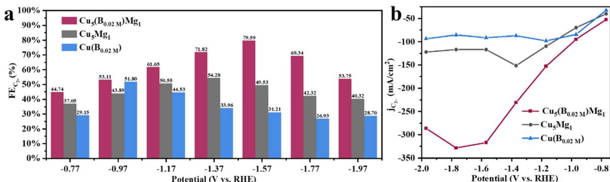
Fig. 5 Electrochemical CO<sub>2</sub>RR performance of the Cu<sub>5</sub>(B<sub>0.02</sub> M)Mg<sub>1</sub> catalyst: (a) FEs of C<sub>2+</sub> (C<sub>2</sub>H<sub>4</sub>, C<sub>2</sub>H<sub>5</sub>OH and CH<sub>3</sub>COOH) at different potentials and (b) partial current densities of C<sub>2+</sub>.
