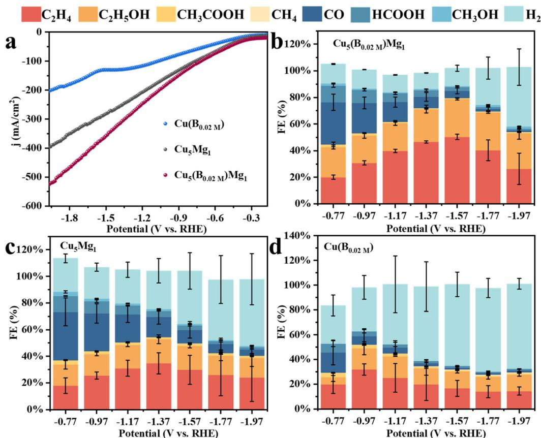
Fig. 4 (a) LSVs of  $\text{Cu}(\text{B}_{0.02\text{ M}})$ ,  $\text{Cu}_5\text{Mg}_1$  and  $\text{Cu}_5(\text{B}_{0.02\text{ M}})\text{Mg}_1$ . The Faraday efficiencies (FEs) of all products for different catalysts: (b)  $\text{Cu}_5(\text{B}_{0.02\text{ M}})\text{Mg}_1$ , (c)  $\text{Cu}_5\text{Mg}_1$ , and (d)  $\text{Cu}(\text{B}_{0.02\text{ M}})$ .
