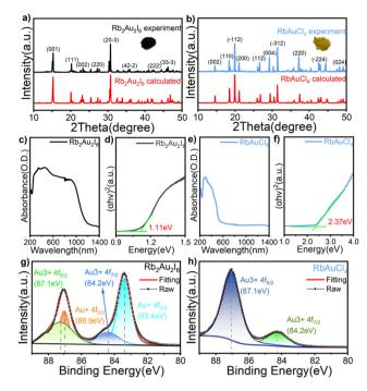
Fig. 2 (a and b) PXRD patterns of Rb<sub>2</sub>Au<sub>2</sub>I<sub>6</sub> and RbAuCl<sub>4</sub> with the calculated XRD patterns of the single crystals; (c and e) powder absorption spectra of Rb<sub>2</sub>Au<sub>2</sub>I<sub>6</sub> and RbAuCl<sub>4</sub>; (d and f) optical bandgaps determined using the Tauc plot formula; and (g and h) XPS spectra in the Au 4f region of Rb2Au2l6 and RbAuCl4. The oxidation state of Au and the position of the fitting peak are indicated in the figure.
