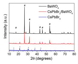
Fig. 7 Experimental XRD patterns of CsPbBr<sub>3</sub>, BaWO<sub>4</sub>, and CsPbBr<sub>3</sub>/ BaWO₄.
