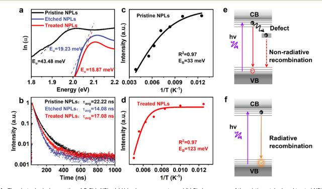
Fig. 4 The photophysical properties of CsPbl<sub>3</sub> NPLs. (a) Urbach energy spectra and (b) PL decay curves of the pristine, etched, and treated NPLs. (c and d) The function and fitting curve of the reciprocal of the PL intensity and temperature for both the pristine and treated NPLs. (e and f) Schematic representations of the PL radiative recombination process for the pristine and treated NPLs.
