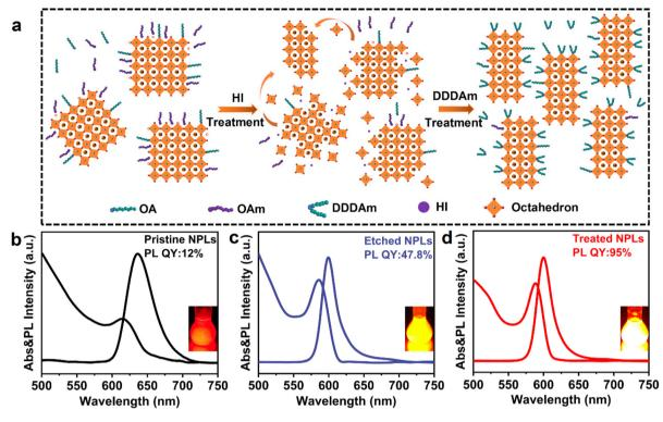
Fig. 1 HI-assisted ligand treatment method for the synthesis of CsPbI<sub>3</sub> NPLs. (a) Schematic outlines the synthesis strategy. (b-d) Absorption and PL spectra of (b) pristine CsPbI<sub>3</sub> NPLs, (c) etched CsPbI<sub>3</sub> NPLs using HI, and (c) treated CsPbI<sub>3</sub> NPLs using HI and the DDDAm ligand. The insets display digital photos of colloidal solutions on these NPLs under 365 nm UV lamp excitation.
