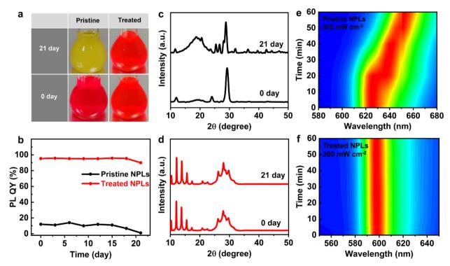
Fig. 5 The stability of CsPbI<sub>3</sub> NPLs. (a) Digital photos of the pristine and treated NPLs before and after 21 days of exposure to environmental conditions, and (b) the corresponding PL QY variation curves. (c and d) XRD patterns of the pristine (c) and treated (d) NPLs before and after 21 days of exposure to environmental conditions. (e and f) 2D pseudo color PL spectral evolution of the pristine (e) and treated (f) NPLs under continuous 365 nm UV light irradiation for 1 h.
