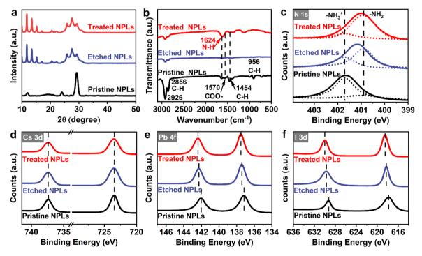
Fig. 3 The microstructure of the pristine, etched, and treated CsPbl<sub>3</sub> NPLs. (a) XRD patterns. (b) FTIR spectra. (c) N 1s, (d) Cs 3d, (e) Pb 4f, and (f) I 3d of XPS spectra.
