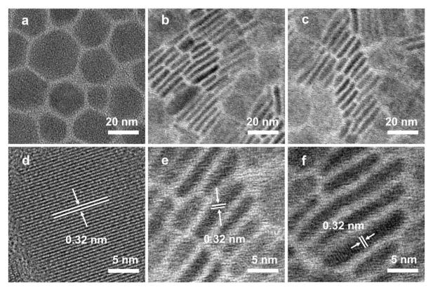
Fig. 2 Morphology of CsPbI<sub>3</sub> NPLs during the HI-assisted ligand treatment process. TEM images of (a) pristine, (b) etched, and (c) treated NPLs. High-resolution TEM images of (d) pristine, (e) etched, and (f) treated NPLs.
