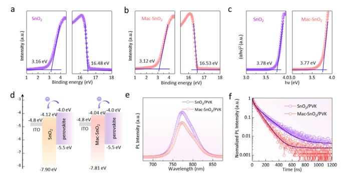
Fig. 5 UPS spectra of (a) SnO<sub>2</sub> and (b) Mac-SnO<sub>2</sub>. (c) Tauc plots of SnO<sub>2</sub> (left) and Mac-SnO<sub>2</sub> (right). (d) Energy band structure diagram of the ETL and perovskite. (e) PL and (f) TRPL spectra of perovskite layers deposited on glass/SnO2 and glass/Mac-SnO2 substrates.
