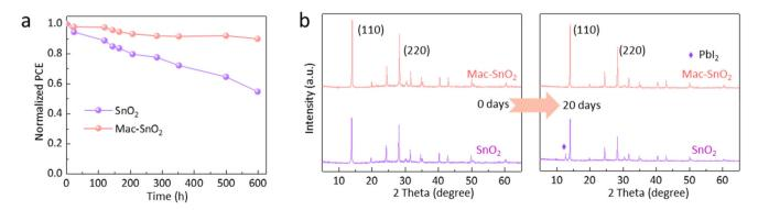
Fig. 7 (a) Normalized PCEs of SnO<sub>2</sub> and Mac-SnO<sub>2</sub> PSCs placed in the ambient environment (25–30 °C, 30%–40% humidity). (b) XRD spectra of the  $SnO_2$ /perovskite and Mac- $SnO_2$ /perovskite before and after exposure to an air environment with 30%-40% humidity for 20 days.
