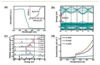
Fig. 3 (a) The UV-vis absorption spectrum of  $\bf 1$  (inset: the experimental bandgap). (b) The calculated bandgap diagram of  $\bf 1$ . (c) PDOS of  $\bf 1$ . (d) Variable temperature conductivity test along different axes of single crystals.
