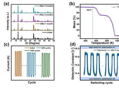
Fig. 5 (a) The phase stability of 1 by the PXRD patterns. (b) TG curve of 1. (c) The photoresponse capability of 1 after 800 and 1200 I-T cycles at 405 nm. (d) Periodic of repeatable switching measurement after several on/off cycles at 1 MHz.
