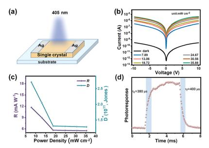
Fig. 4 (a) The photodetection device schematic diagram of 1. (b) The I-V curves of 1 measured at 405 nm with different incidence powers. (c) R and D\* calculated from the photocurrent measured at 10 V bias. (d) The response time of 1.
