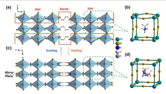
Fig. 1 (a) A schematic diagram of the quantum-well-like structure of 1 at LTP. (b) The inorganic framework, with the MA<sup>+</sup> cation incorporated inside the cavity at LTP. (c) Single crystal structures of 1 at HTP. (d) The inorganic framework, with the disordered MA+ cation inside the cavity at HTP; the two folds of cations have been distinguished in different colours.
