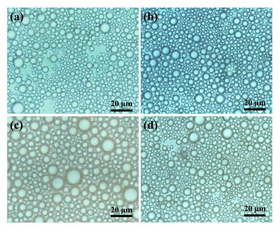
Fig. 5 Optical microscopy images of the emulsions prepared using toluene as the oil phase: PEG-b-PLA as the surfactant after storing for (a) 24 h and (c) 7 d, and PA-g-PFA/PEG/PLA as the surfactant after storing for (b) 24 h and (d) 7 d.
