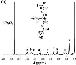
Fig. 1 <sup>1</sup>H NMR spectra of (a) the Br-acrylate-epoxide functional monomer and (b) the poly(Br-acrylate-epoxide) macro-agent.
