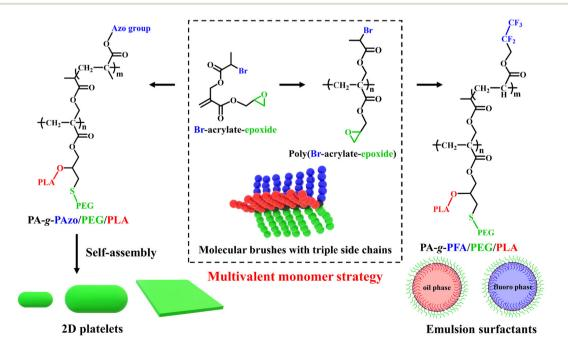
Scheme 1 Chemical structures of the multivalent monomer Br-acrylate-epoxide, the macro-agent poly(Br-acrylate-epoxide), and the asymmetric molecular brushes with triple side chains PA-q-PAzo/PEG/PLA and PA-q-PFA/PEG/PLA. Schematic representations of the self-assembly behavior of PA-g-PAzo/PEG/PLA and the surfactant properties of PA-g-PFA/PEG/PLA.
