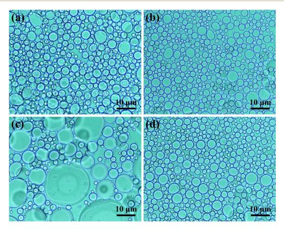
Fig. 6 Optical microscopy images of the emulsions prepared using hexafluorobenzene as the oil phase: PEG-b-PFA as the surfactant after storing for (a) 24 h and (c) 7 d, and PA-g-PFA/PEG/PLA as the surfactant after storing for (b) 24 h and (d) 7 d.
