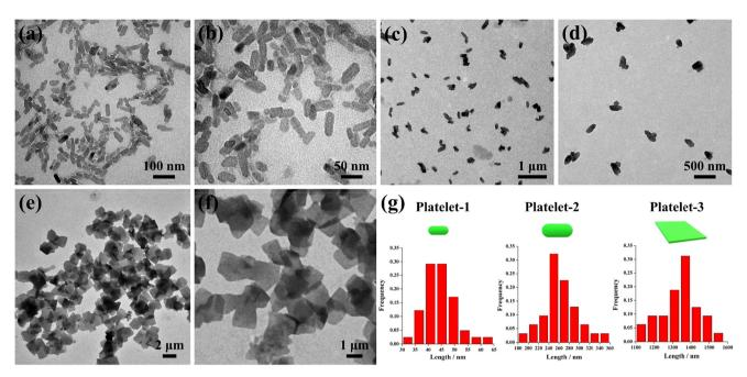
Fig. 3 TEM images of 2D platelets formed by PA-g-PAzo/PEG/PLA in a mixture of CH $_3$ OH and THF ( $V_{\rm methanol}$ :  $V_{\rm THF}$  = 92 : 8) with concentrations of (a, b) 0.015 mg mL $^{-1}$ , platelet-1, (c, d) 0.02 mg mL $^{-1}$ , platelet-2, and (e, f) 0.04 mg mL $^{-1}$ , platelet-3. (g) Statistical analysis of the length distribution of the platelets.
