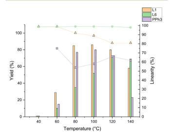
Fig. 2 Influence of temperature in hydroformylation of 1a for selected ligands. Conditions: olefin (6.0 mmol), [Rh(CO)<sub>2</sub>acac] (0.014 mol%), monodentate ligand (0.071 mol%), CO:H<sub>2</sub> (10 bar, 1:1), toluene (4.3 mL), 4 h. The yield and regioselectivity of the product were measured by GC analysis using MeOH as solvent and isooctane as internal standard.
