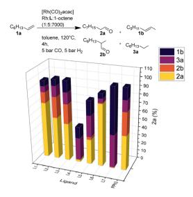
Fig. 3 Influence of ligands in hydroformylation of 1a. in optimized conditions. Conditions: 1a (6.0 mmol), [Rh(CO)2acac] (0.014 mol%), monodentate ligand (0.071 mol%), CO: H2 (10 bar, 1:1), toluene (4.3 mL), 120 °C, 4 h. The conversion of 1a and yields of 2a, 2b, 1b, 3a and regioselectivity of the products were measured by GC analysis using MeOH as solvent and isooctane as internal standard.
