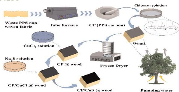
**Solar-driven water evaporation using a collaborative photothermal conversion material system based on carbonized waste polyphenylene sulfide and copper sulfide**
